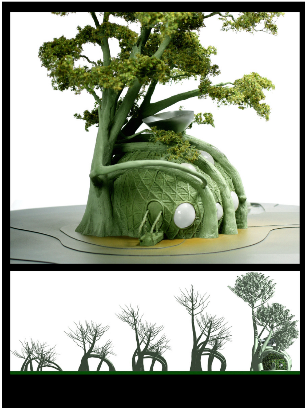
Mitchell Joachim and colleagues at Terreform ONE developed the Fab Tree Hab, shown here as a 3-D model (top), to demonstrate that a home could be composed entirely of living materials. The renderings (bottom) show the Fab Tree Hab's progression of growth. Image: Courtesy of Mitchell Joachim, Terreform ONE
